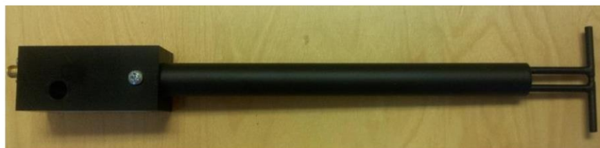
Figure 1 – MVG COMOSAR Validation Dipole
