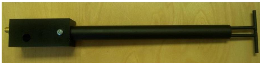
Figure 1 – MVG COMOSAR Validation Dipole
