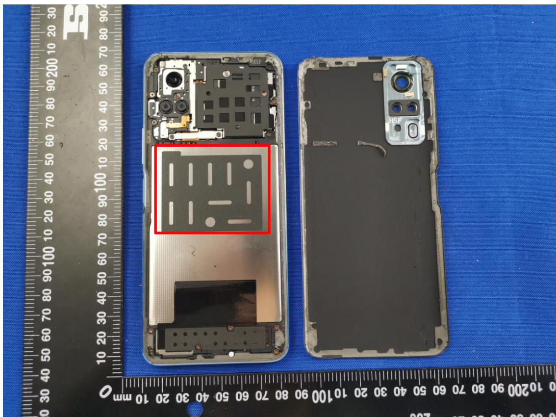
EUT UNCOVER VIEW_BATTERY COVER WITH FOAM GASKET
