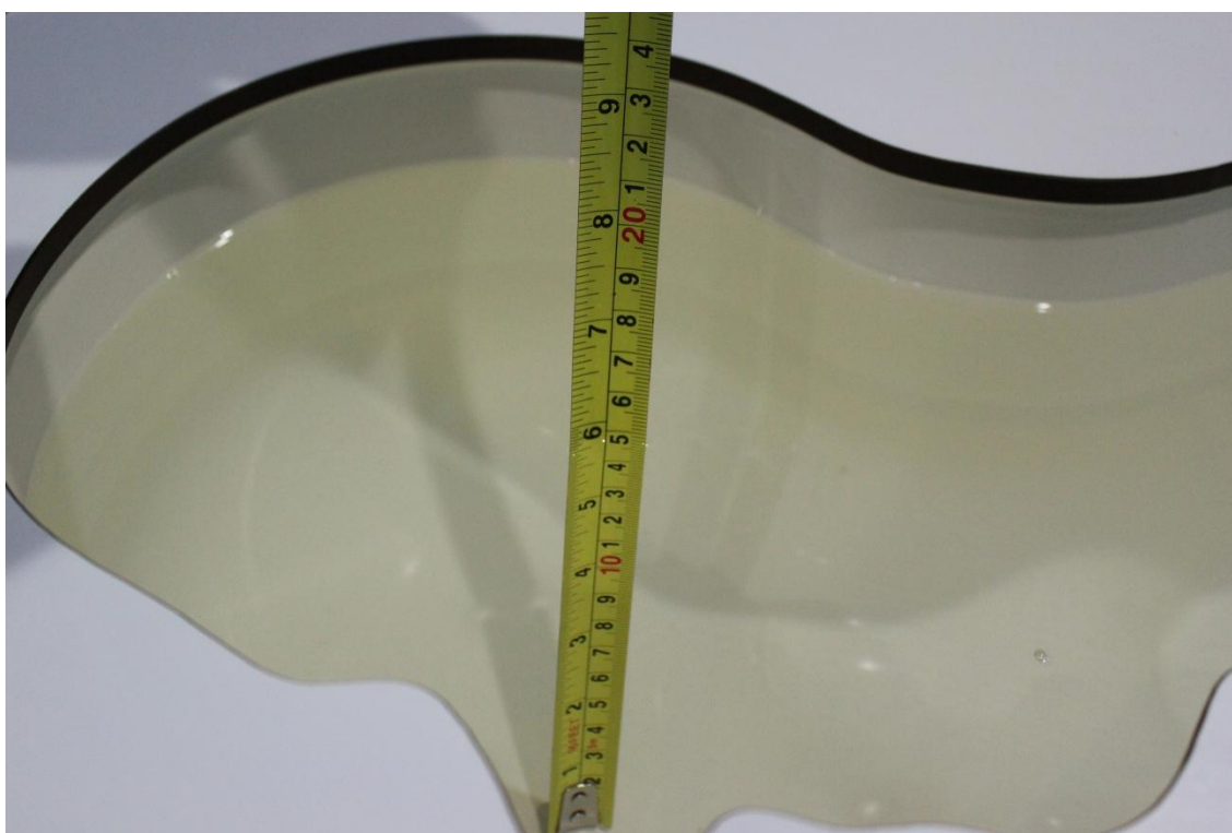
Picture 7-8 Liquid depth in the Head Phantom (5GHz)
