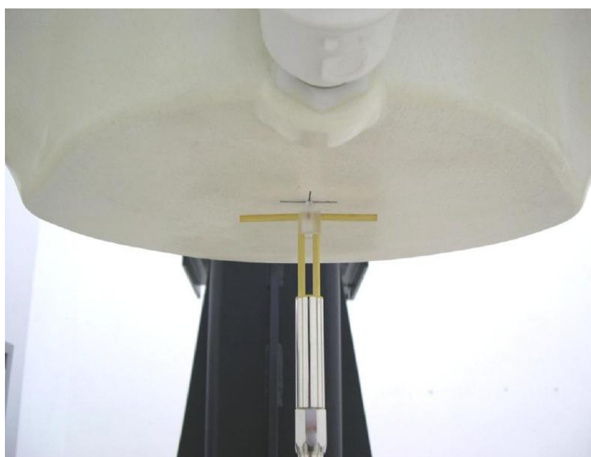
Picture 8.2 Photo of Dipole Setup
