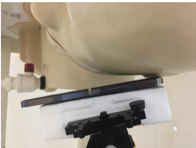
Left Tilted, Test Separation 0 mm
