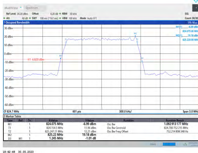
Band26-1.4MHz-QPSK-26915-6RB#0
