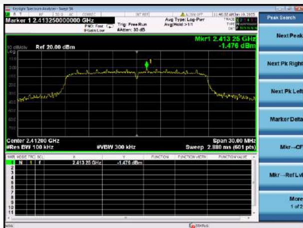
VHT-20 MHz LOW CHANNEL, CARRIER LEVEL
