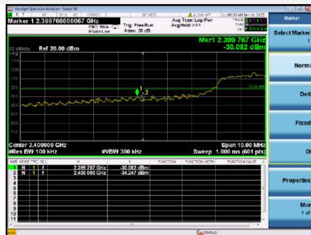
VHT-20 MHz LOW CHANNEL, BAND EDGE
