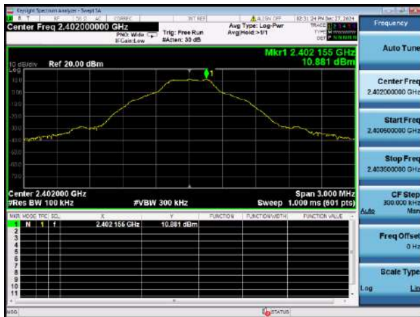
GFSK LOW CHANNEL, CARRIER LEVEL
