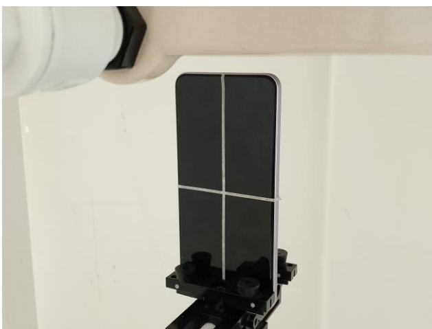
Bottom Side, Test Separation 10 mm
