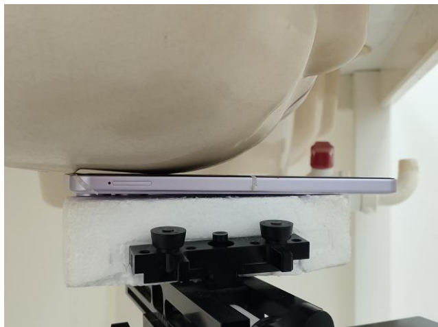
Right Cheek, Test Separation 0 mm
