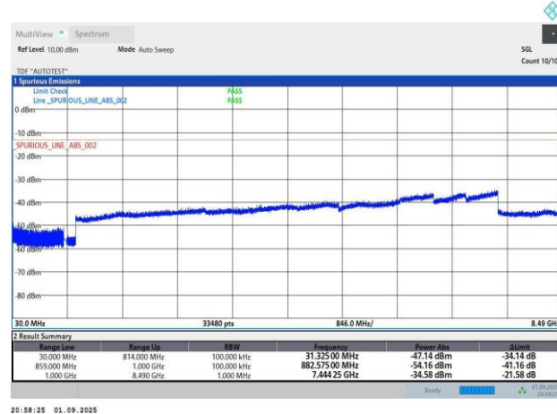
Band26-10MHz-QPSK-26840-1RB#0-PASS
