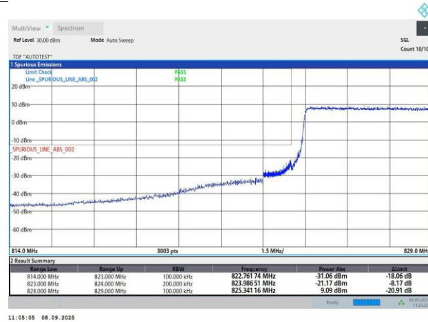
Band26-10MHz-QPSK-26840-25RB#0-PASS
