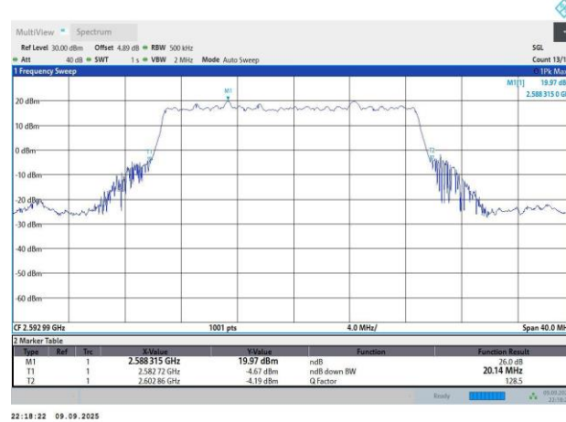
N41-30KHz-20MHz-DFT-s-OFDM PI/2 BPSK-518598-50RB#0-18.12-20.14
