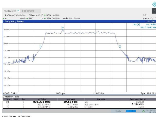
N5-15KHz-5MHz-DFT-s-OFDM PI/2 BPSK-167300-25RB#0-4.52-5.16
