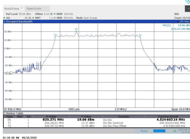
N5-15KHz-5MHz-DFT-s-OFDM PI/2 BPSK-167300-25RB#0-4.52-5.16
