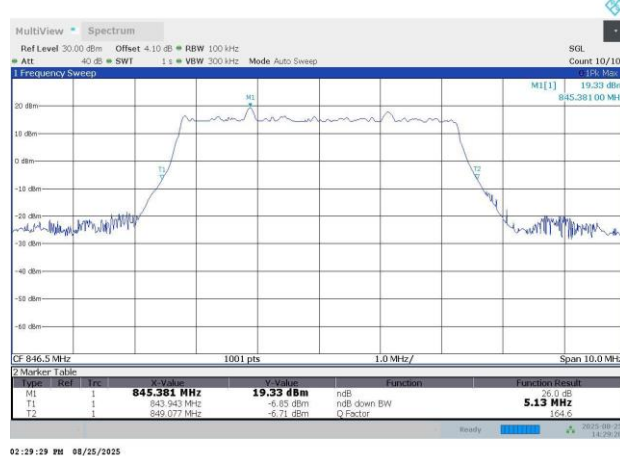
N5-15KHz-5MHz-DFT-s-OFDM PI/2 BPSK-169300-25RB#0-4.53-5.13
