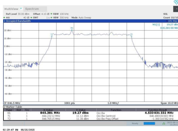
N5-15KHz-5MHz-DFT-s-OFDM PI/2 BPSK-169300-25RB#0-4.53-5.13
