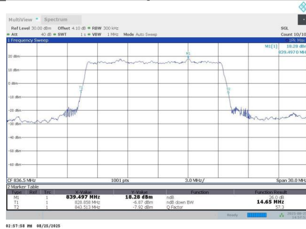
N5-15KHz-15MHz-DFT-s-OFDM PI/2 BPSK-167300-75RB#0-13.47-14.65
