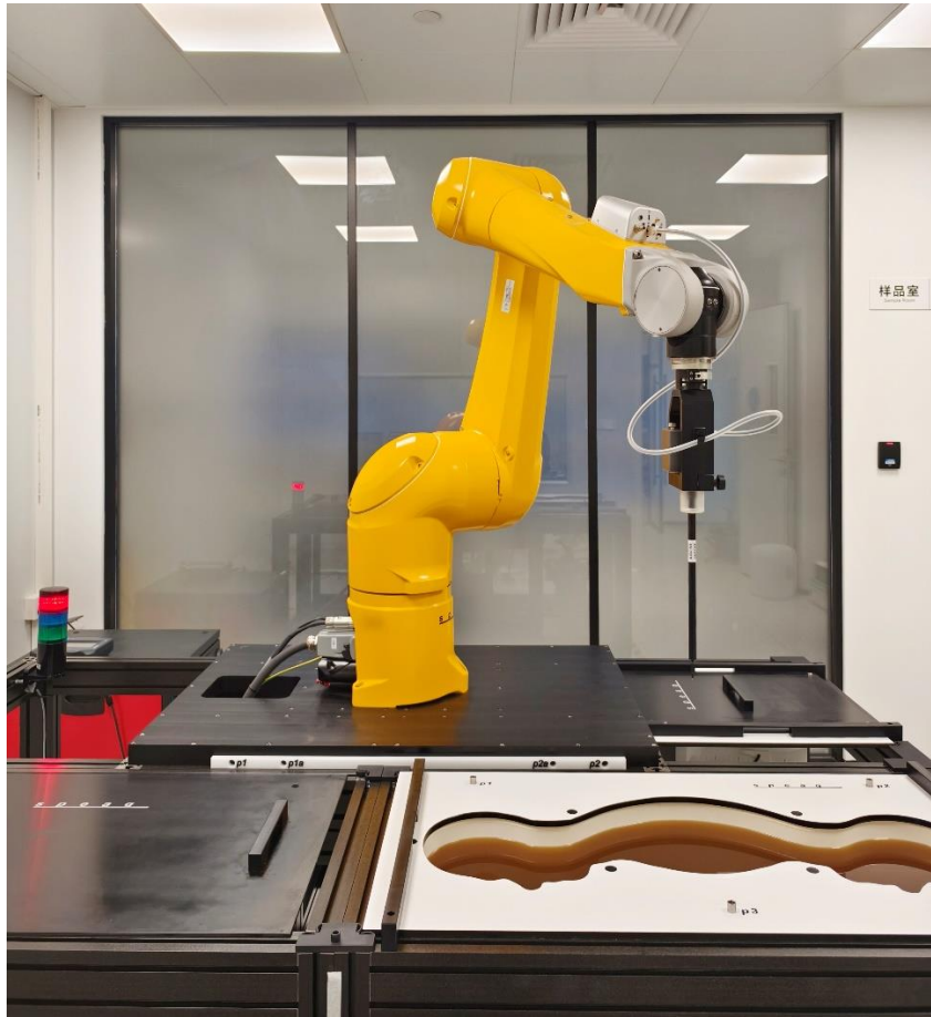
Photo 1: DASY sar measurement system
