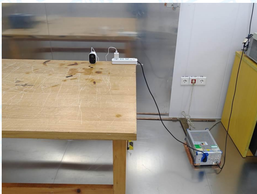
Photo of Setup for Conducted Emission
