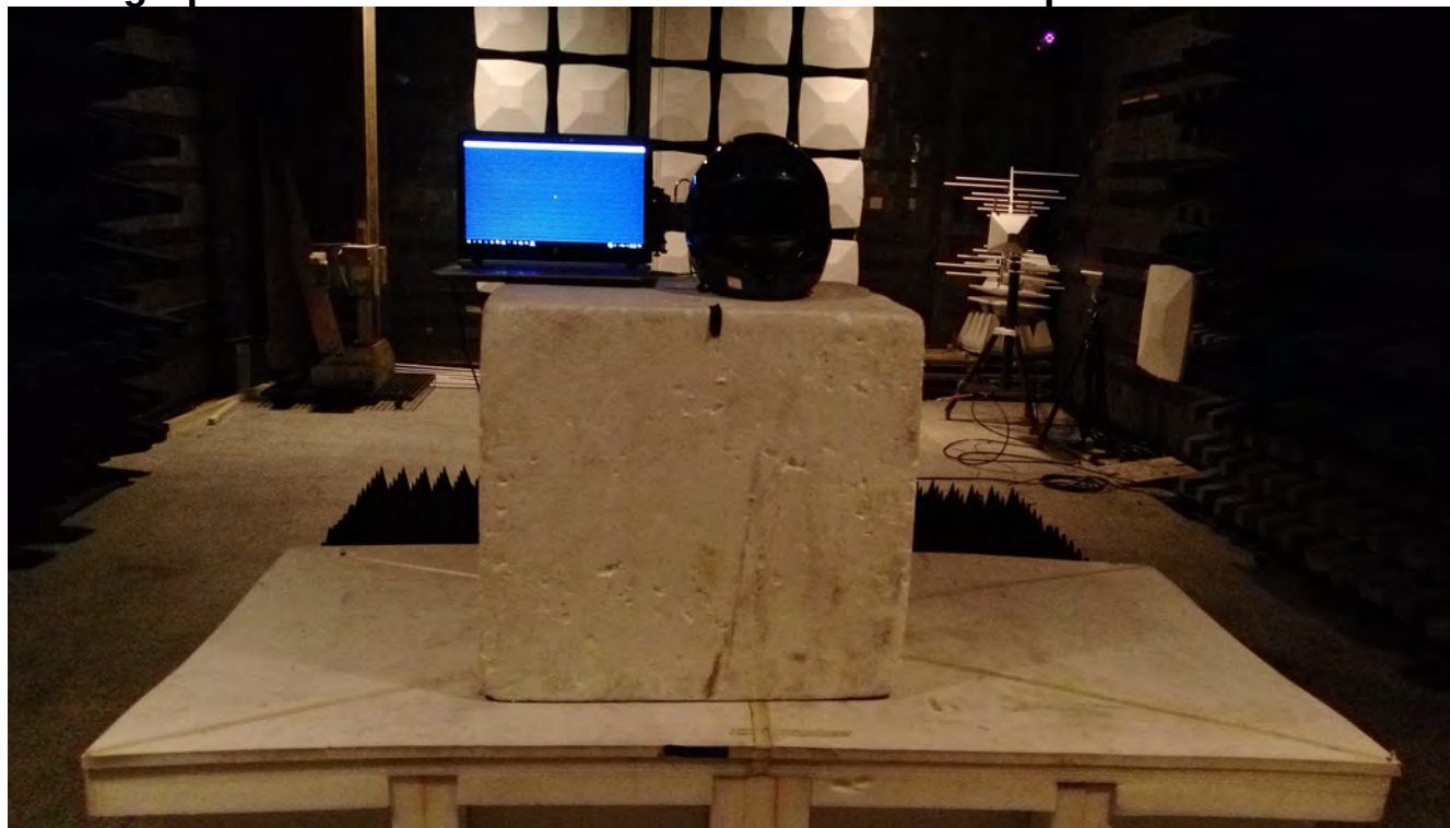
Photograph – Radiated Emission Above 1G Test Setup
