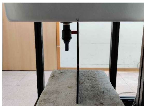
Fig.7 EUT Left side to flat phantom
