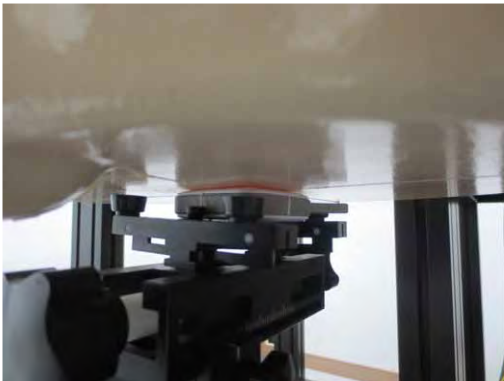
Rear from Flat Phantom (Separation Distance: 0 cm)
