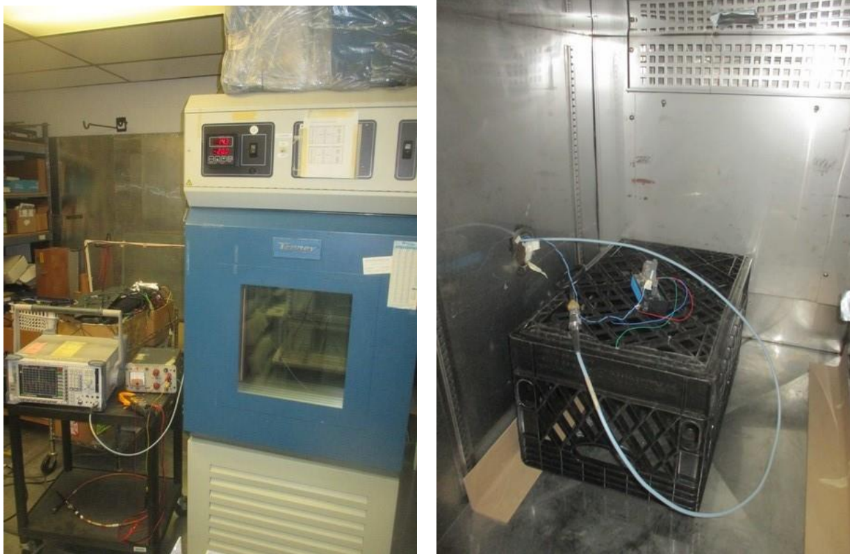
Figure 3.4 Frequency Tolerance Test Setup
