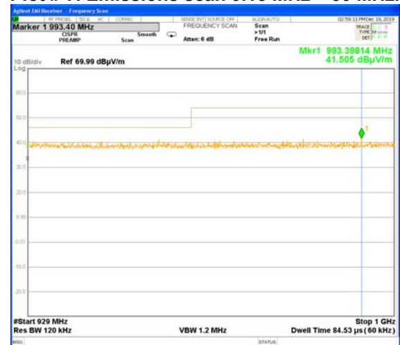
Plot # 9. Emissions scan 929 - 1000 MHz.
