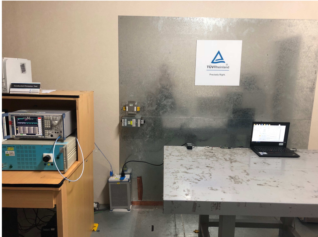
Photograph 6: Set-up for for Mains Conducted testing Front
