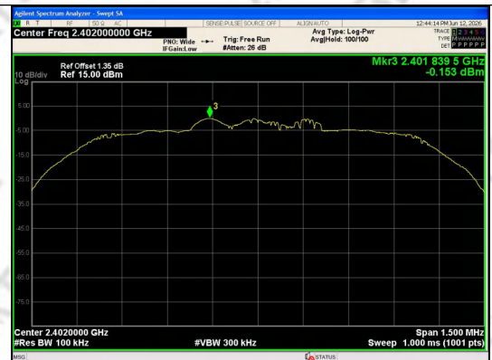
In-Band Reference Level \pi/4 DQPSK 2-DH5 Channel 0
