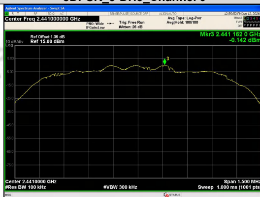
Out Of Band Emission 8DPSK_3-DH5_Channel 0
