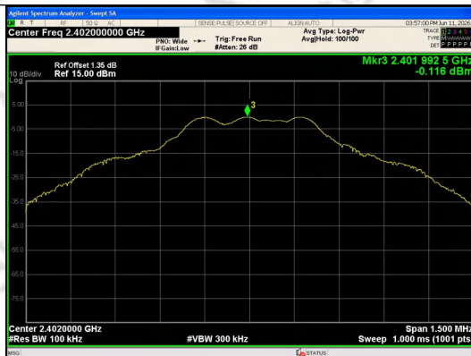
In-Band Reference Level GFSK DH5 Channel 0
