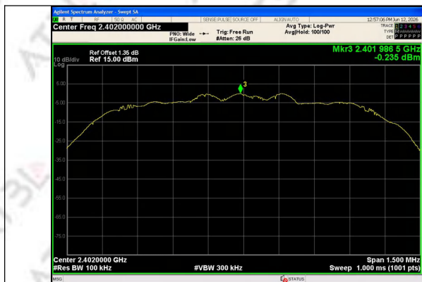
In-Band Reference Level 8DPSK_3-DH5_Channel 0
