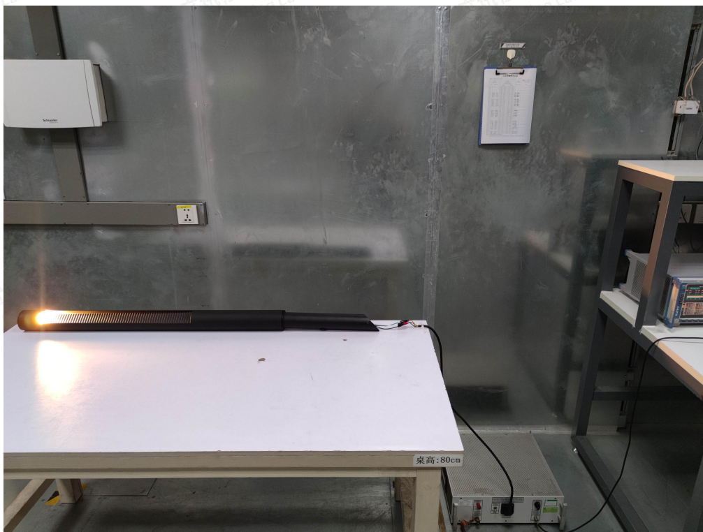
Photo of Power Line Conducted Measurement
