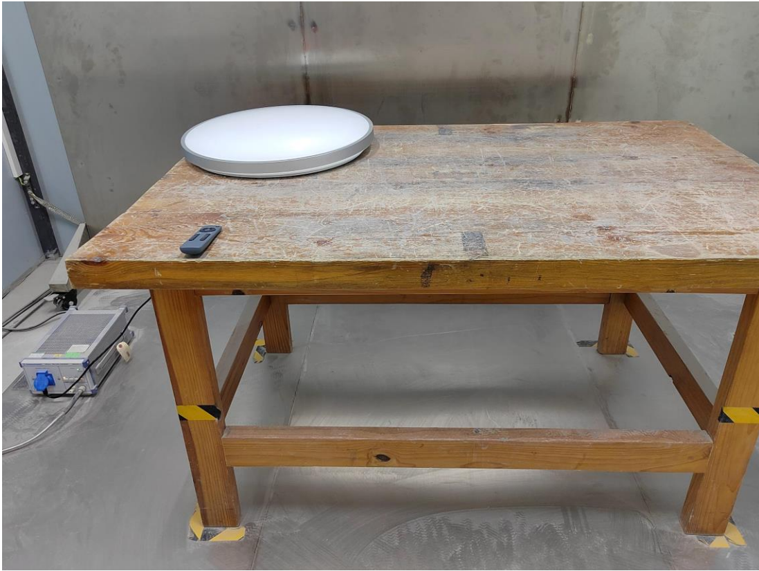
Conducted Emissions Side View
