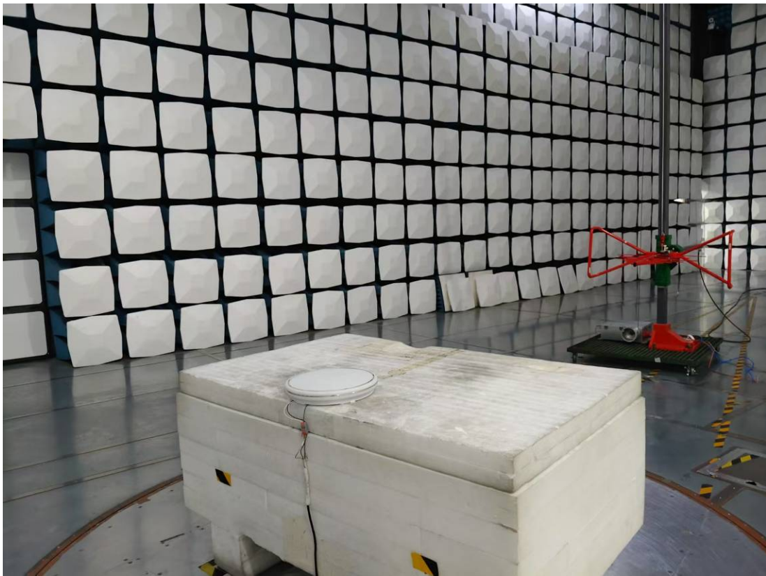
Radiated Emission 30MHz -1GHz Rear View
