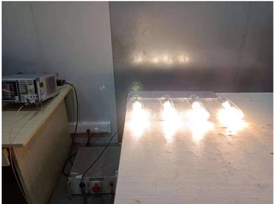
Conducted Emission Test Setup
