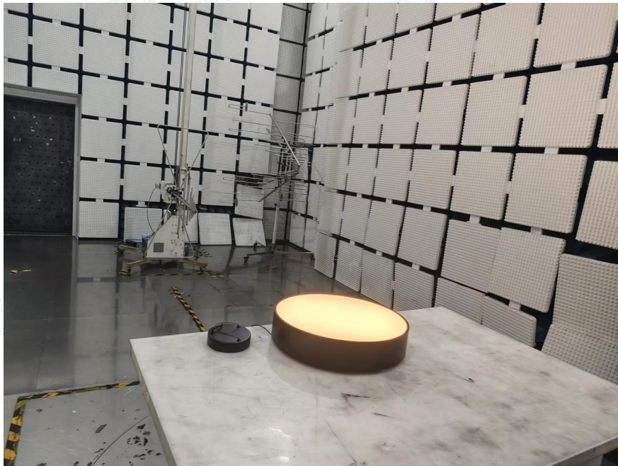
Radiated emissions (Below 1GHz)
