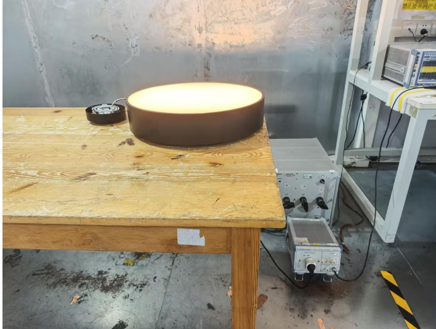
Conducted emissions on AC mains
