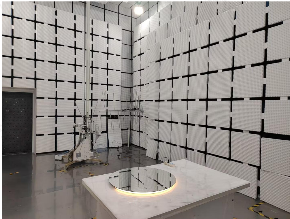
Radiated Emissions Measurement (Below 1GHz)
