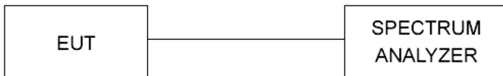
Figure 1 - Bandwidth Measurements Test Setup
