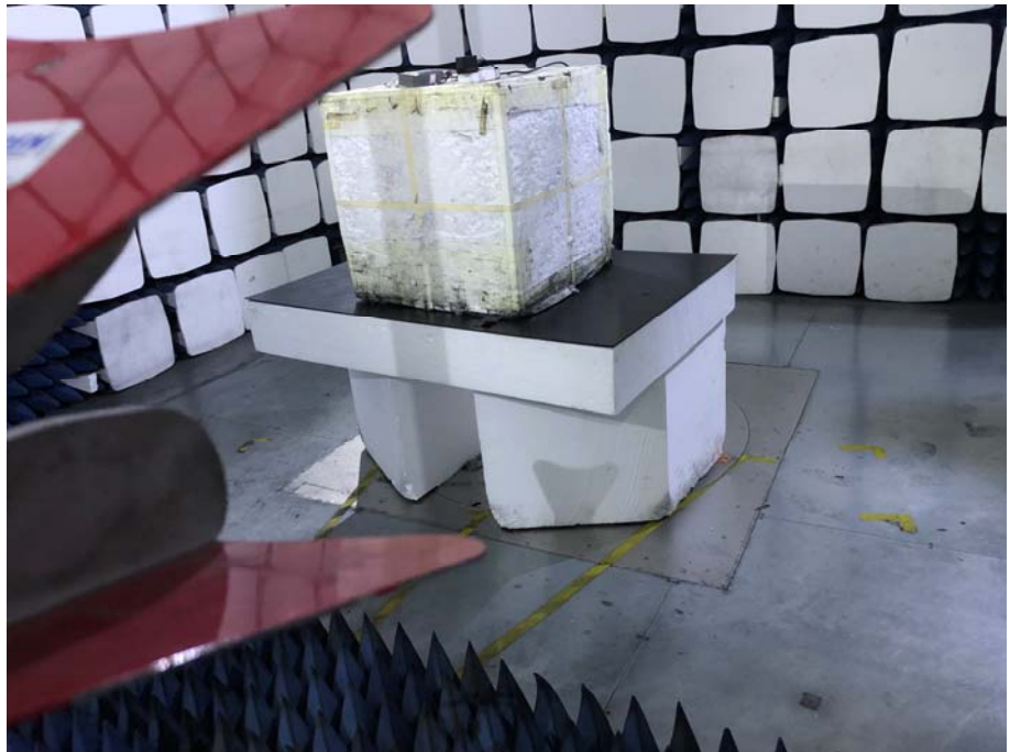
Radiation Emission Test Setup (1GHz to 18GHz)
