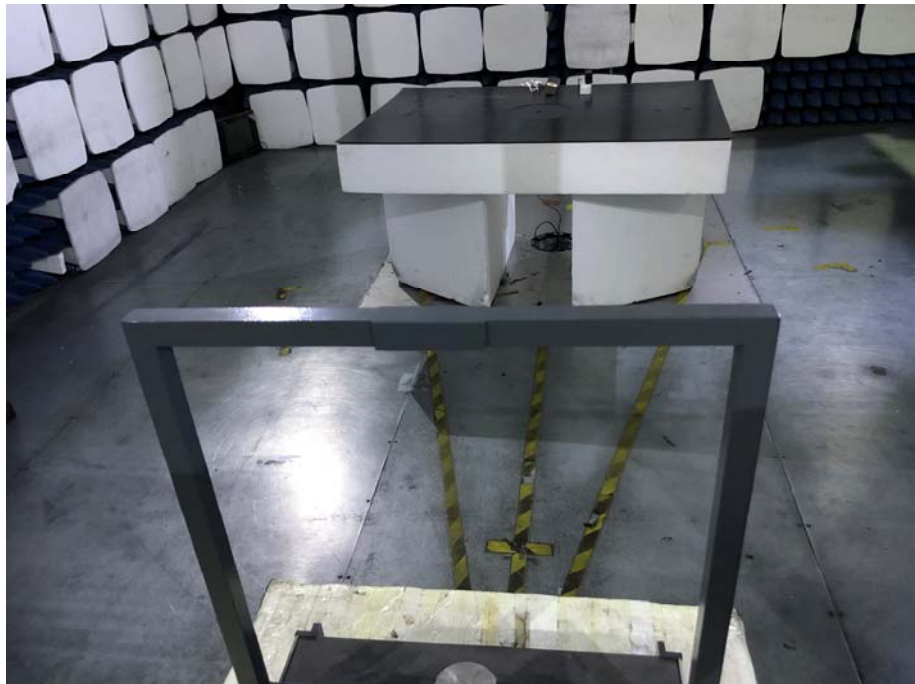
Radiation Emission Test Setup (Below 30MHz)
