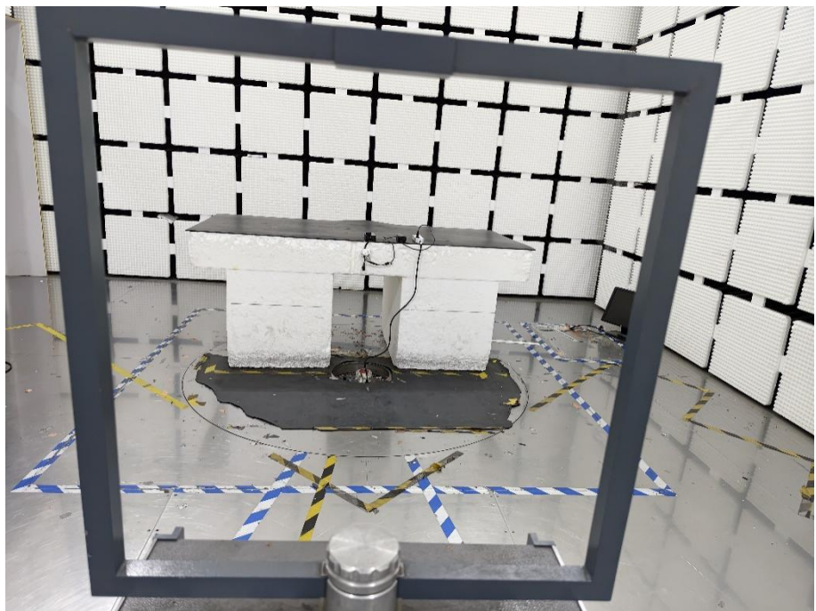
Radiation Emission Test Setup (Below 30MHz)
