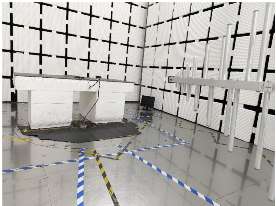
Radiation Emission Test Setup (30MHz to 1GHz)
