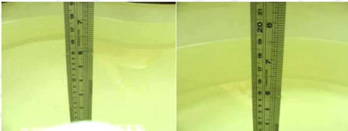
Photo of Liquid Height for Head SAR
