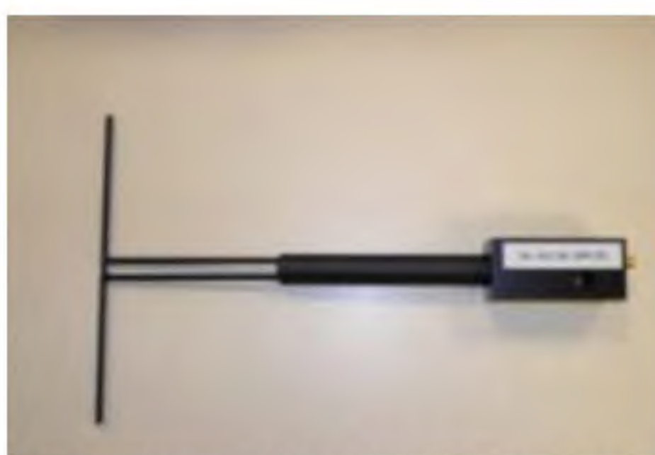
Figure 1 – Satimo COMOSAR Validation Dipole
