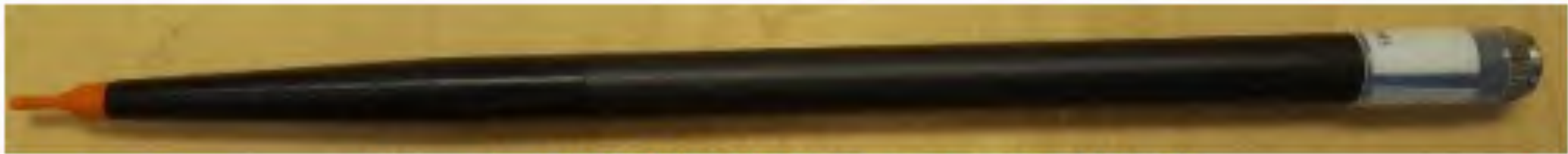
Figure 1 – MVG COMOSAR Dosimetric E field Probe
