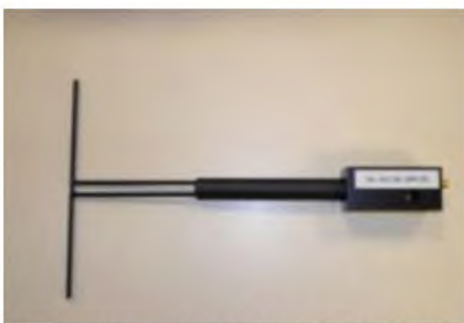
Figure 1 – Satimo COMOSAR Validation Dipole
