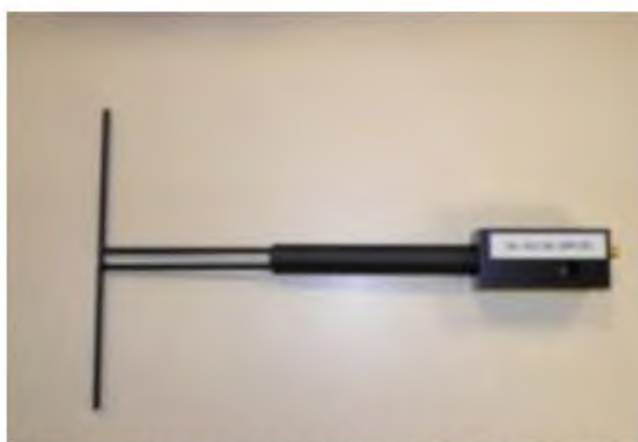
Figure 1 – Satimo COMOSAR Validation Dipole
