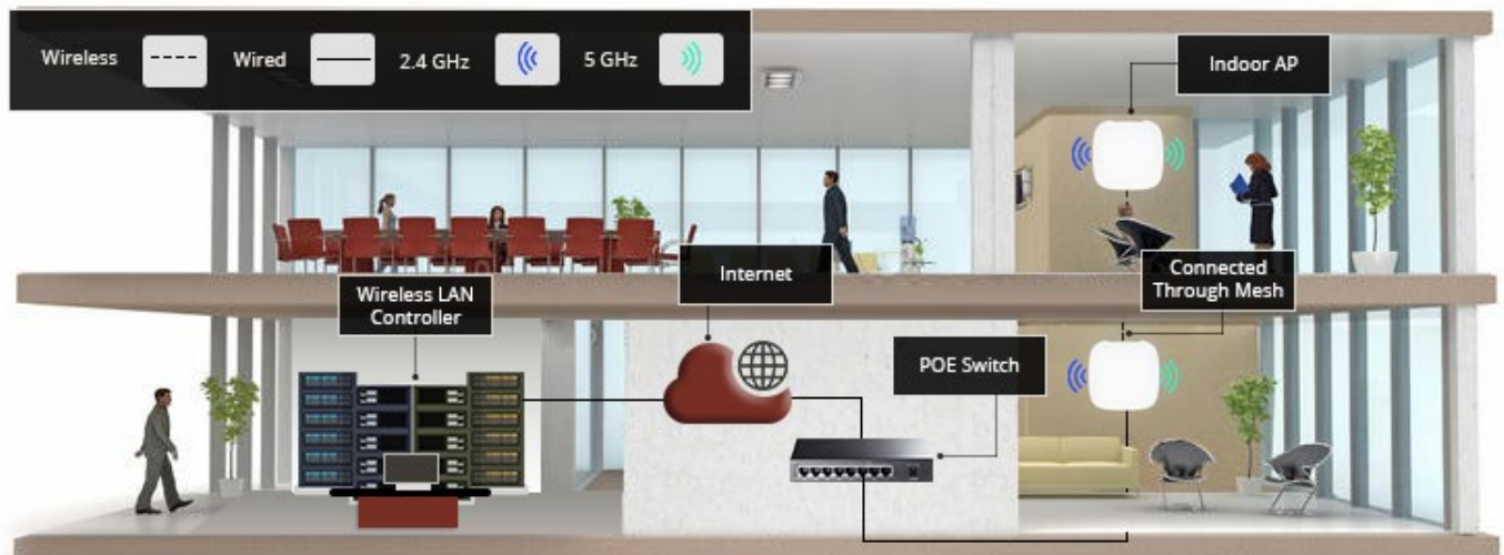
Figure 87: Use Case Diagram of Indoor AP
