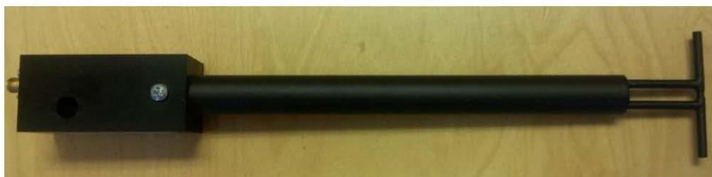
Figure 1 – MVG COMOSAR Validation Dipole
