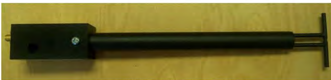
Figure 1 – MVG COMOSAR Validation Dipole
