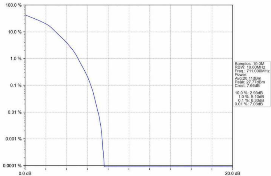
Band12 10MHz 16QAM HCH 711MHz RB 27 23 NTNV
