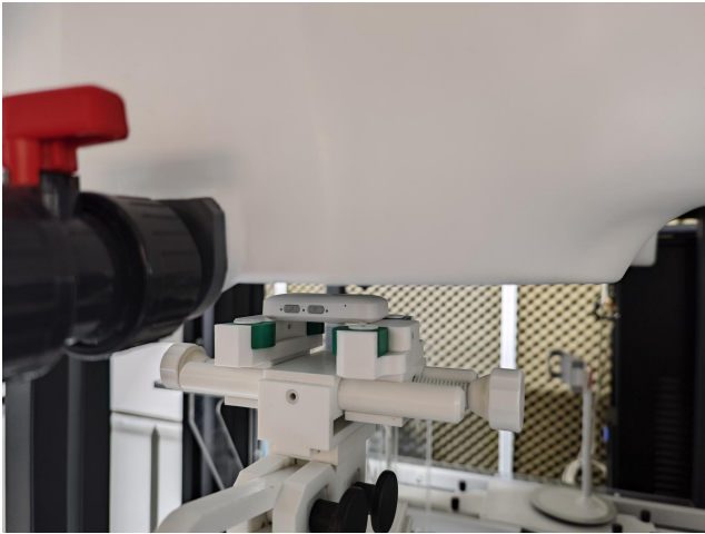
Body-worn Front (dist. 10mm)
