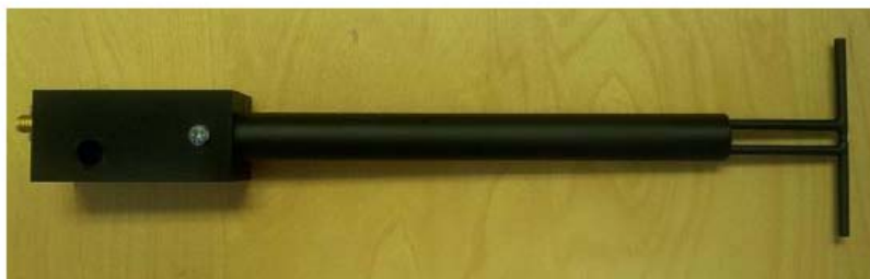
Figure 1 – MVG COMOSAR Validation Dipole
