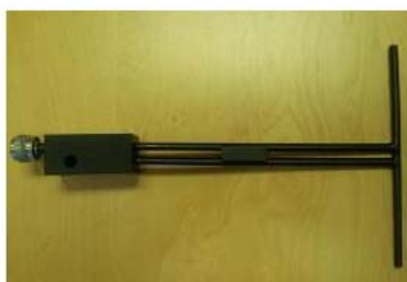
Figure 1 – MVG COMOSAR Validation Dipole
