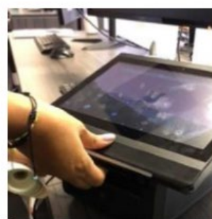
(3) Lift up on paper retainer to expose the paper bucket. (4) Insert thermal paper as shown. (5) Close lid.
