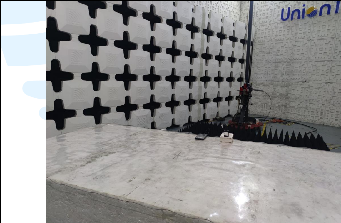
Radiated emission Test Setup-2 (Above 1 GHz) - Test Mode 2
