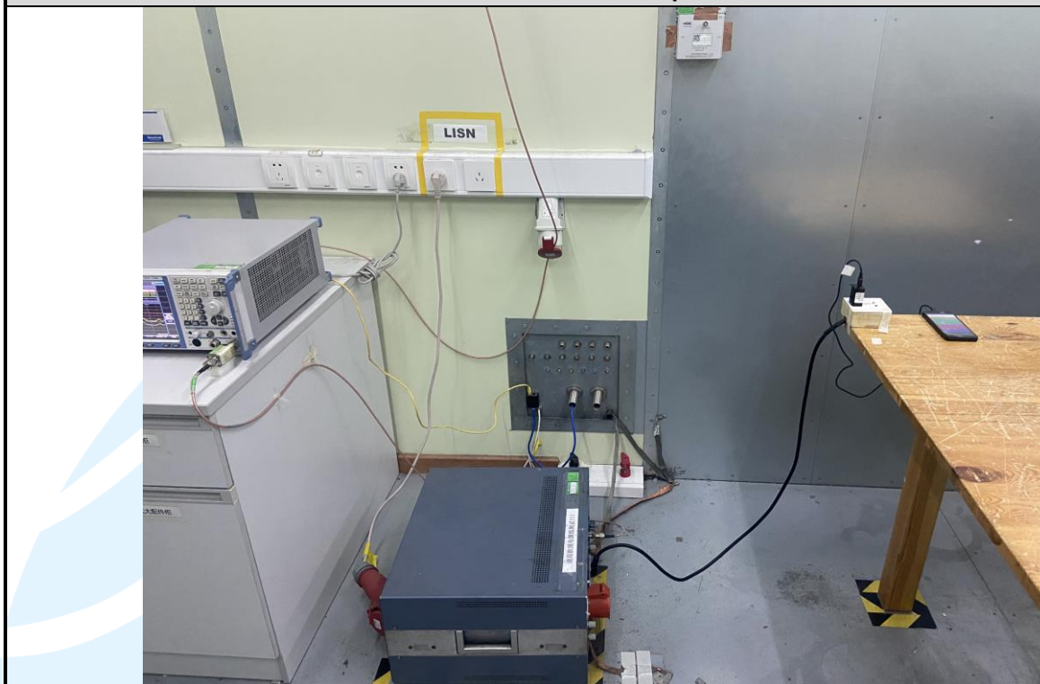
Conducted Emission Test Setup-3 – Test Mode 1
