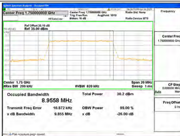
Band4 / 10MHz / 16QAM/ High CH
