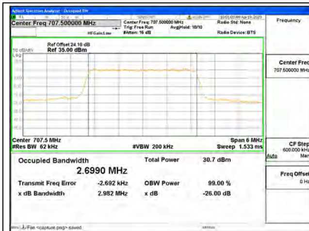
Band12 / 3MHz / QPSK/ Mid CH
