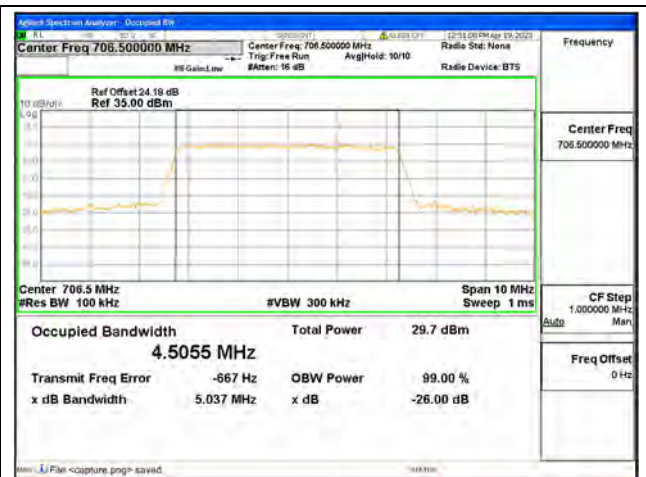
Band17 / 5MHz / 16QAM/ Low CH
