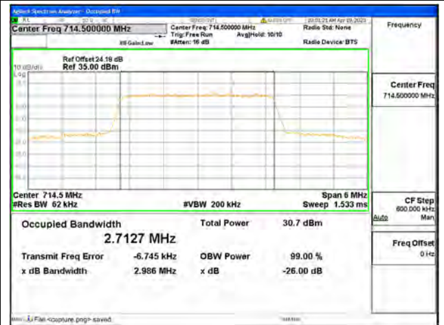
Band12 / 3MHz / QPSK/ High CH
