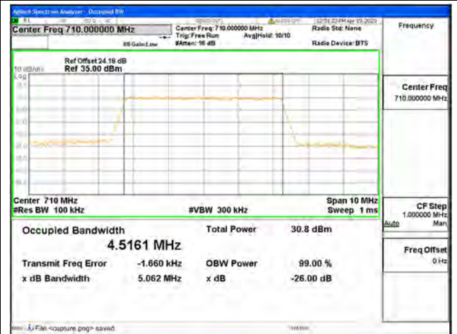
Band17 / 5MHz / QPSK/ Mid CH
