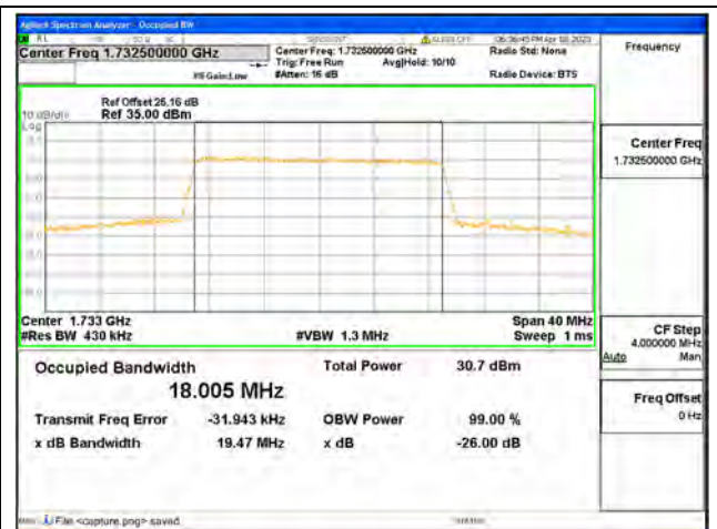
Band4 / 20MHz / 16QAM/ Mid CH
