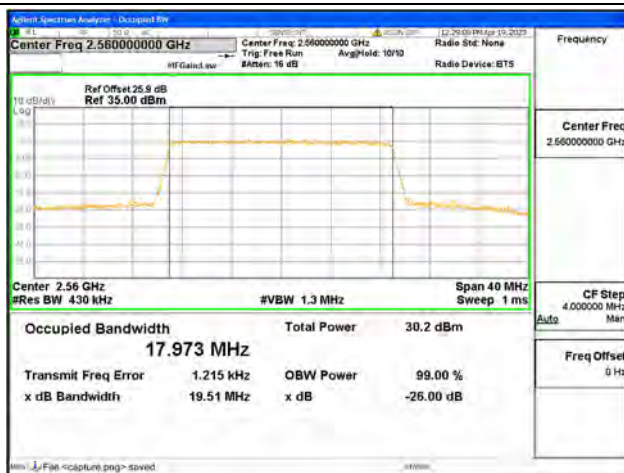
Band7 / 20MHz / 16QAM/ High CH
