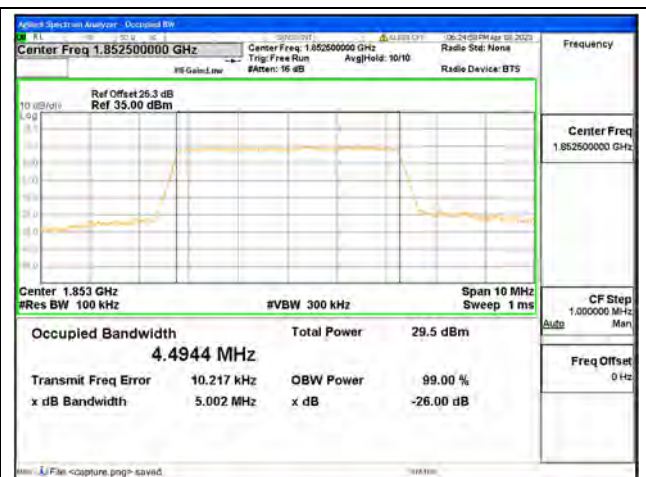
Band2 / 5MHz / 16QAM/ Low CH
