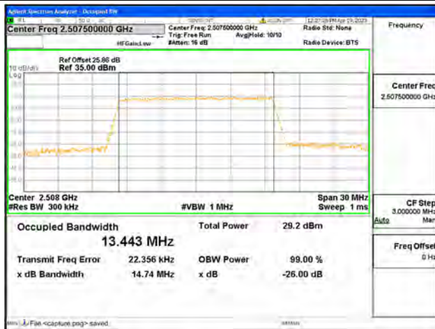
Band7 / 15MHz / 64QAM/ Low CH
