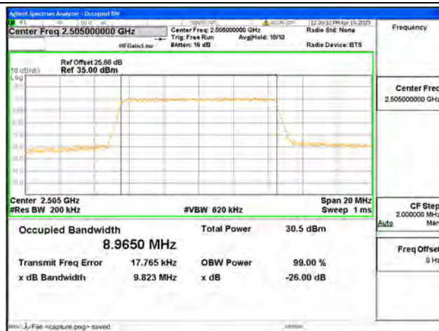
Band7 / 10MHz / 16QAM/ Low CH
