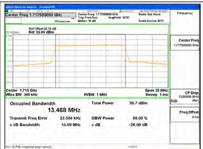
Band4 / 15MHz / 16QAM/ Low CH
