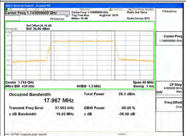
Band4 / 20MHz / 64QAM/ High CH
