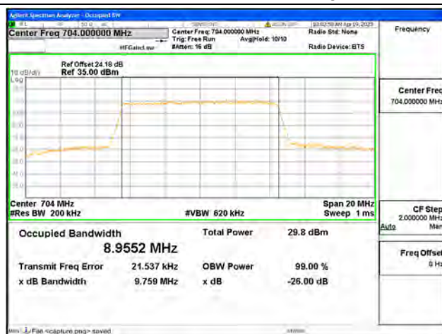
Band12 / 10MHz / 16QAM/ Low CH
