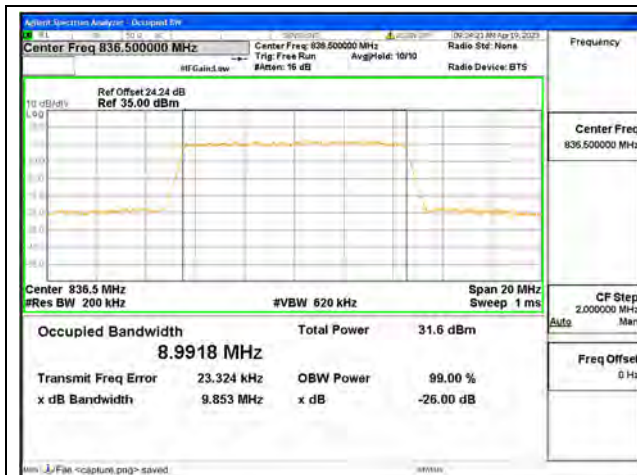
Band5 / 10MHz / QPSK/ Mid CH
