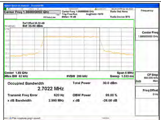
Band2 / 3MHz / 16QAM/ Mid CH
