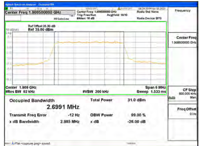
Band2 / 3MHz / QPSK/ High CH
