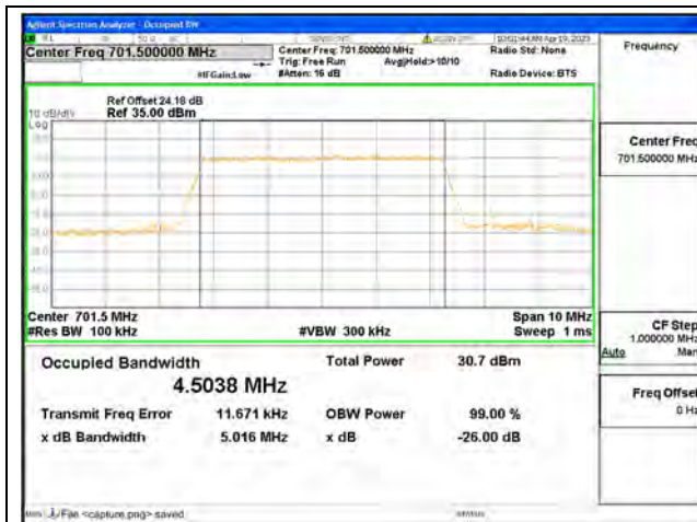
Band12 / 5MHz / QPSK/ Low CH
