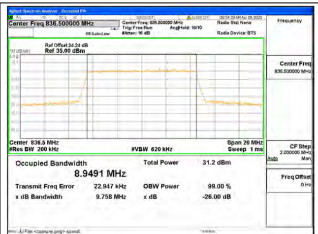
Band5 / 10MHz / 16QAM/ Mid CH
