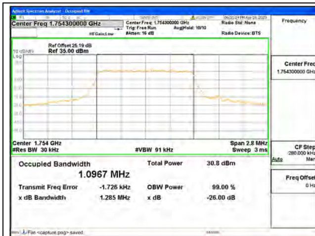
Band4 / 1.4MHz / QPSK/ High CH
