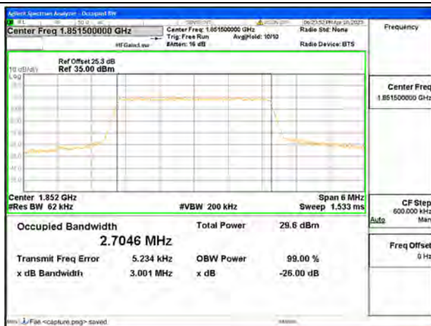
Band2 / 3MHz / 16QAM/ Low CH
