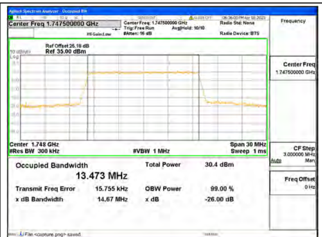
Band4 / 15MHz / 16QAM/ High CH
