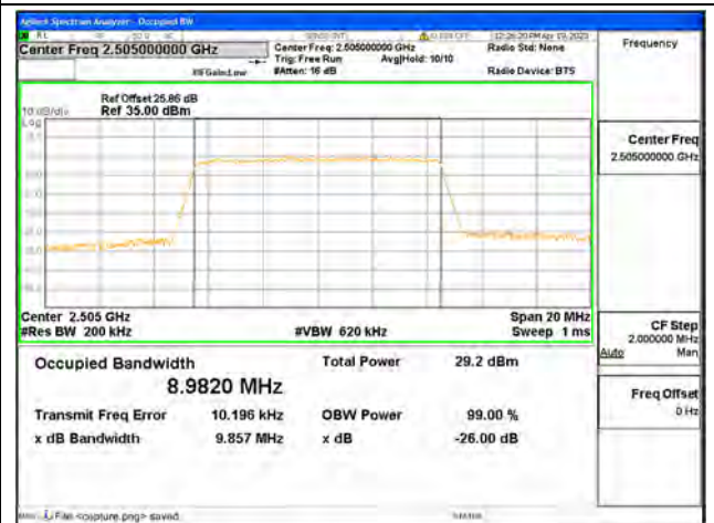
Band7 / 10MHz / 64QAM/ Low CH
