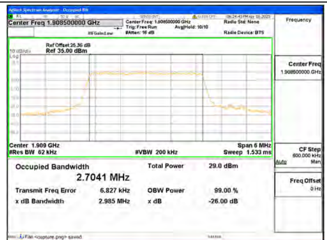
Band2 / 3MHz / 64QAM/ High CH
