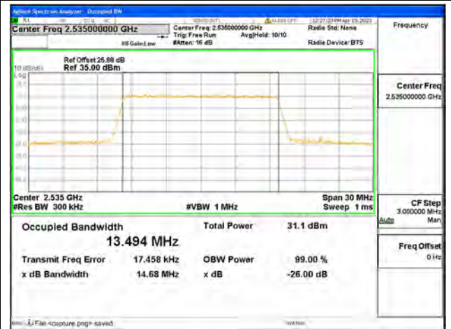
Band7 / 15MHz / QPSK/ Mid CH
