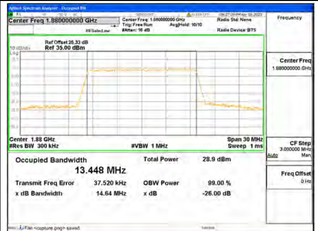
Band2 / 15MHz / 64QAM/ Mid CH
