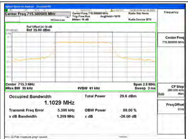
Band12 / 1.4MHz / 16QAM/ High CH
