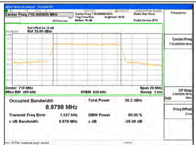
Band17 / 10MHz / 16QAM/ Mid CH
