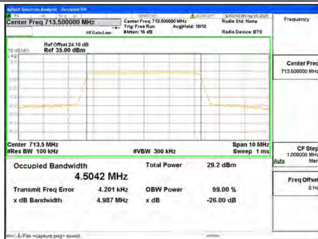
Band12 / 5MHz / 64QAM/ High CH
