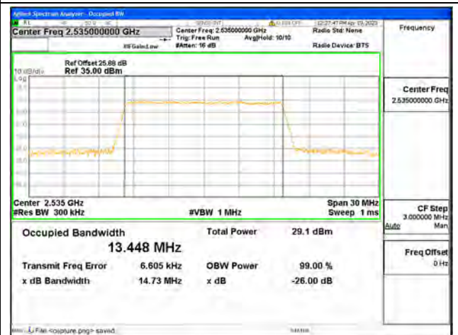
Band7 / 15MHz / 64QAM/ Mid CH
