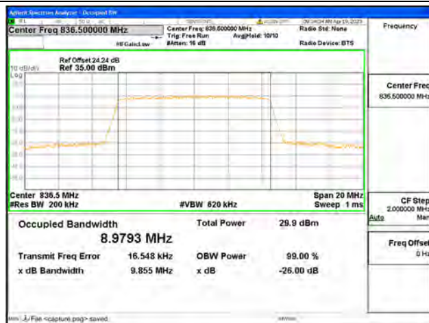
Band5 / 10MHz / 64QAM/ Mid CH
