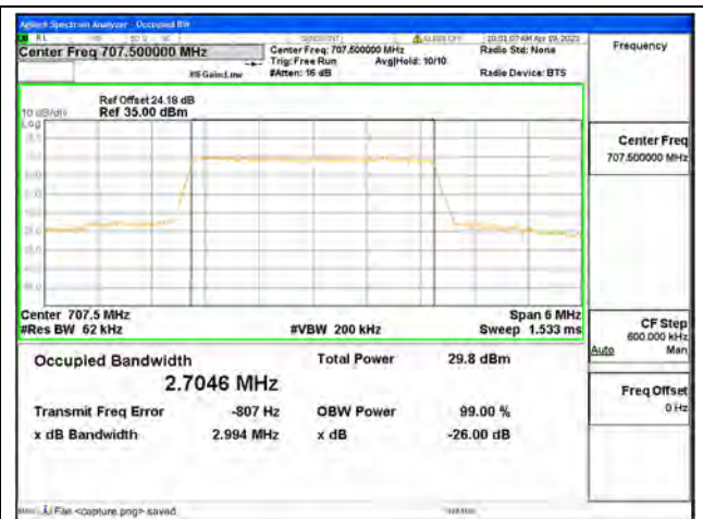
Band12 / 3MHz / 16QAM/ Mid CH
