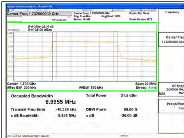
Band4 / 10MHz / QPSK/ Mid CH
