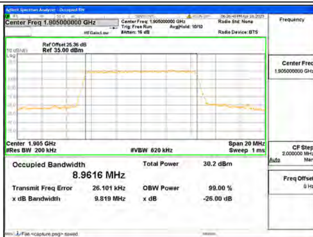
Band2 / 10MHz / 16QAM/ High CH
