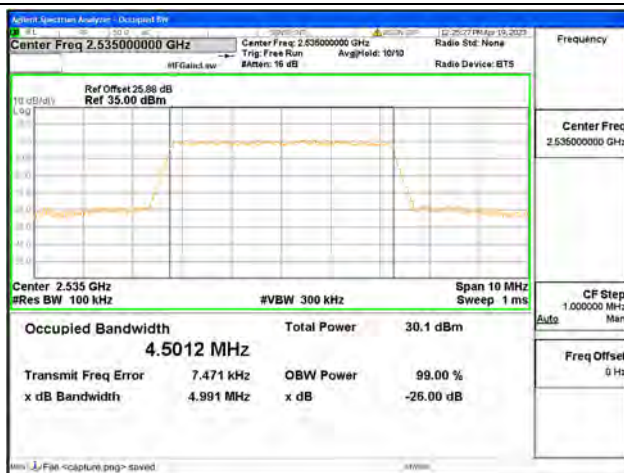
Band7 / 5MHz / 16QAM/ Mid CH
