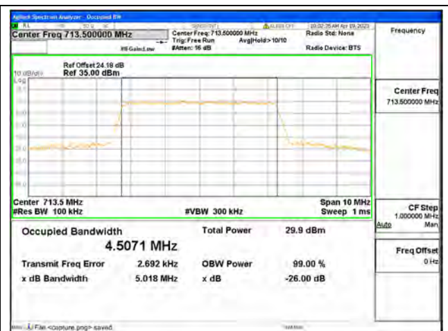
Band12 / 5MHz / 16QAM/ High CH
