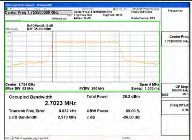
Band4 / 3MHz / 64QAM/ High CH
