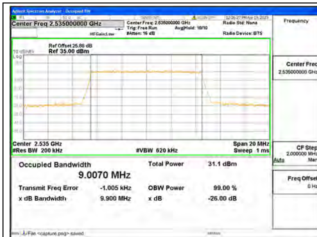
Band7 / 10MHz / QPSK/ Mid CH
