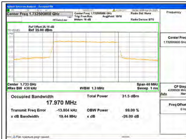
Band4 / 20MHz / QPSK/ Mid CH
