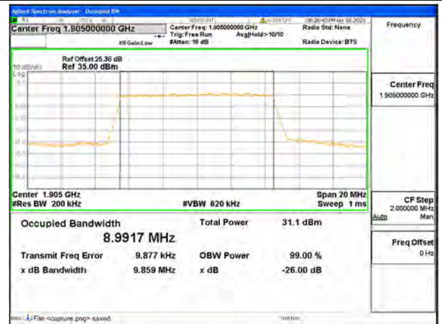
Band2 / 10MHz / QPSK/ High CH
