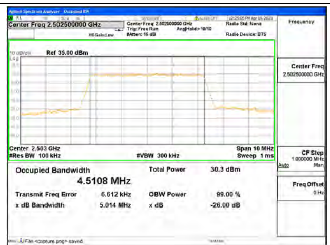
Band7 / 5MHz / 16QAM/ Low CH
