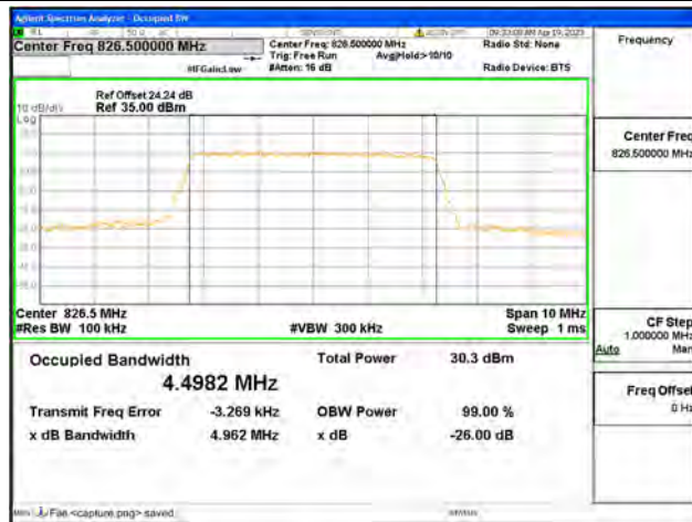
Band5 / 5MHz / 64QAM/ Low CH
