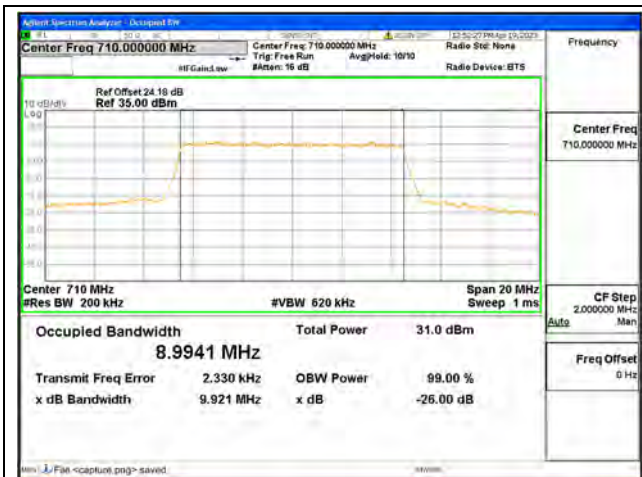
Band17 / 10MHz / QPSK/ Mid CH
