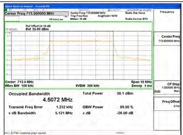
Band17 / 5MHz / 16QAM/ High CH
