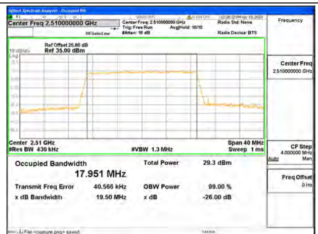
Band7 / 20MHz / 64QAM/ Low CH
