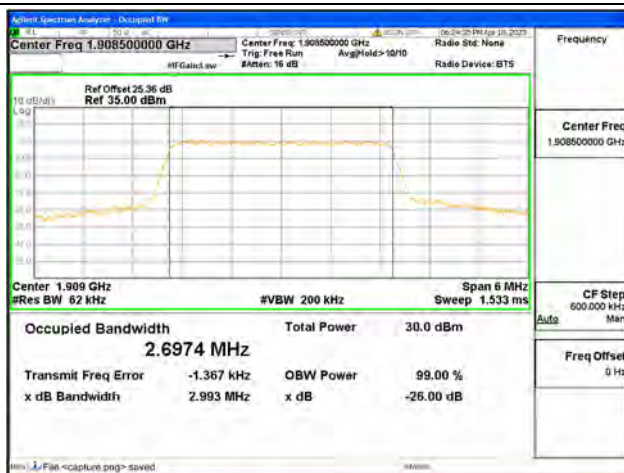
Band2 / 3MHz / 16QAM/ High CH
