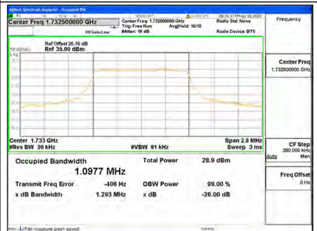
Band4 / 1.4MHz / 64QAM/ Mid CH
