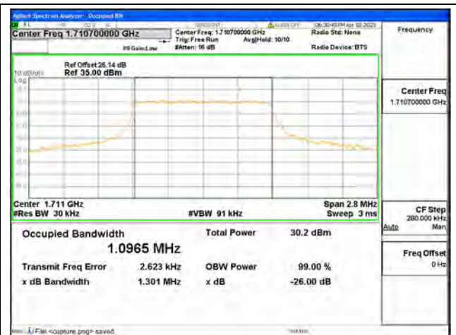
Band4 / 1.4MHz / 16QAM/ Low CH
