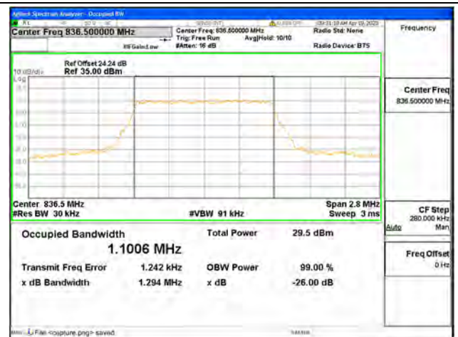
Band5 / 1.4MHz / 64QAM/ Mid CH
