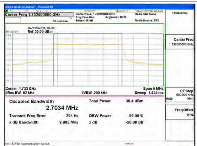
Band4 / 3MHz / 16QAM/ Mid CH
