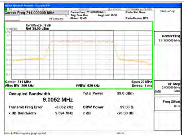
Band17 / 10MHz / 64QAM/ High CH
