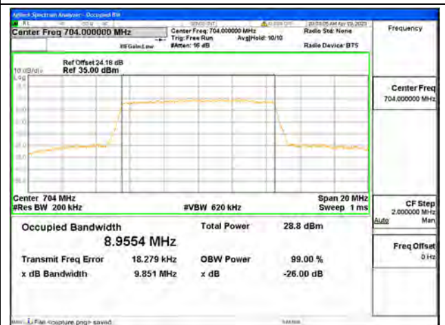
Band12 / 10MHz / 64QAM/ Low CH
