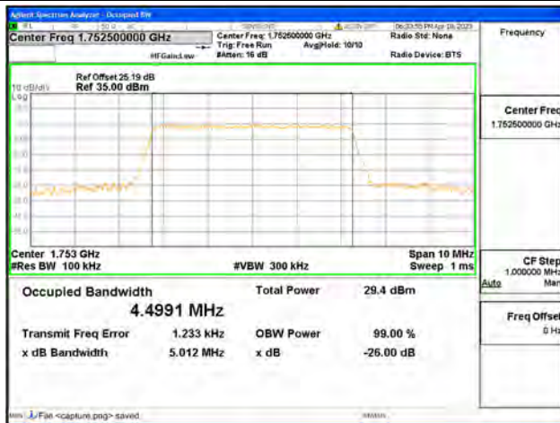
Band4 / 5MHz / 64QAM/ High CH
