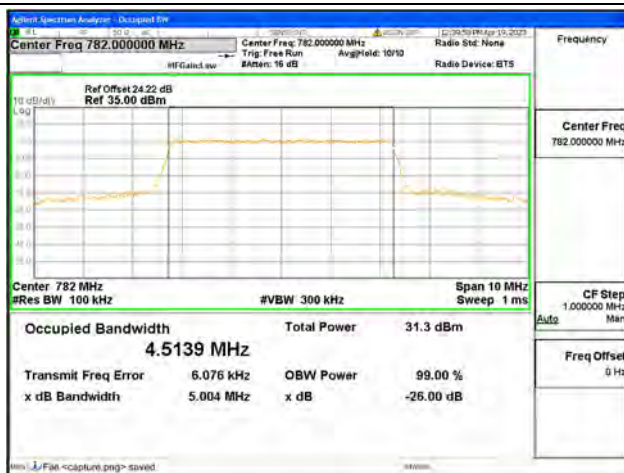
Band13 / 5MHz / 16QAM/ Mid CH
