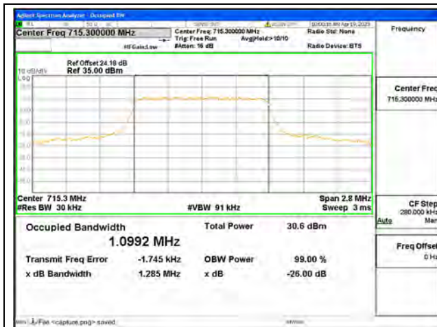
Band12 / 1.4MHz / QPSK/ High CH
