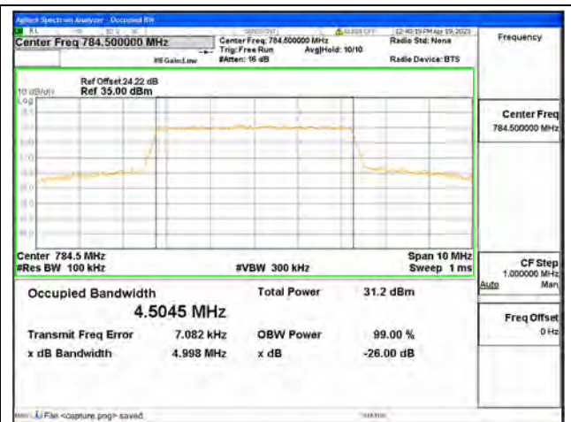
Band13 / 5MHz / 16QAM/ High CH
