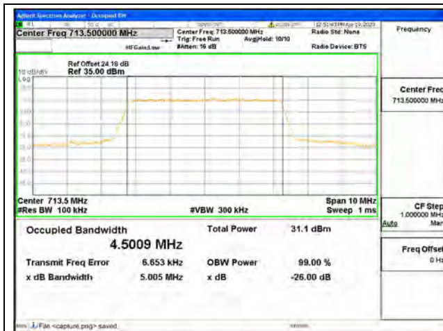
Band17 / 5MHz / QPSK/ High CH
