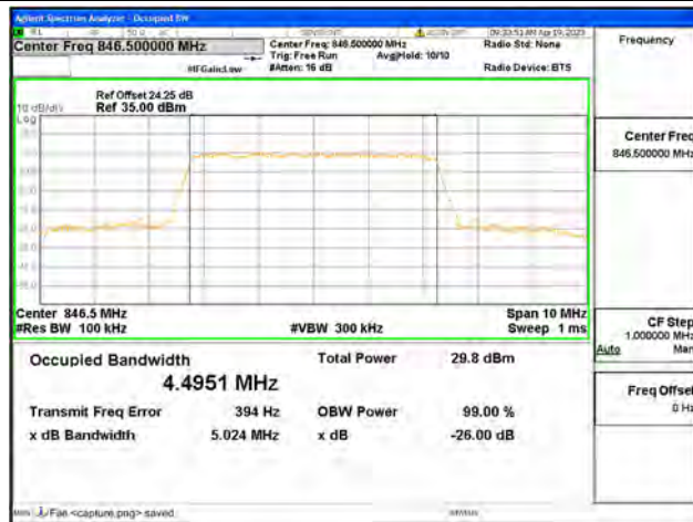
Band5 / 5MHz / 64QAM/ High CH
