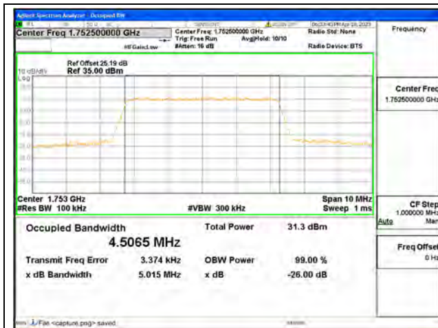
Band4 / 5MHz / QPSK/ High CH
