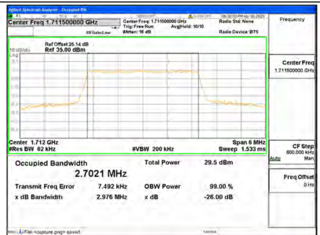
Band4 / 3MHz / 64QAM/ Low CH
