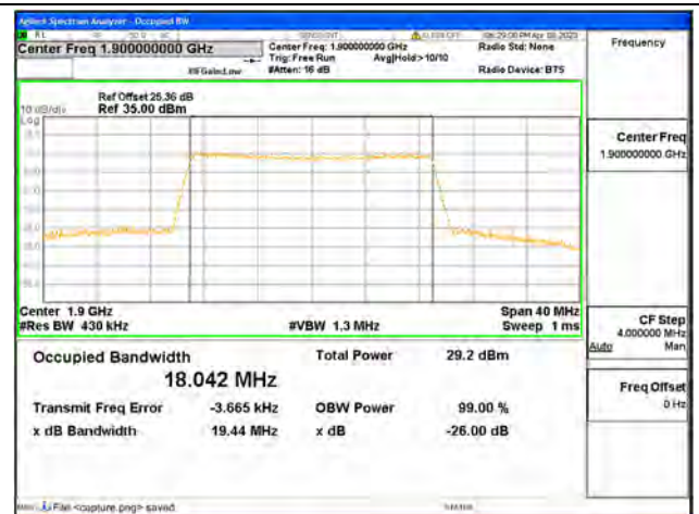
Band2 / 20MHz / 64QAM/ High CH
