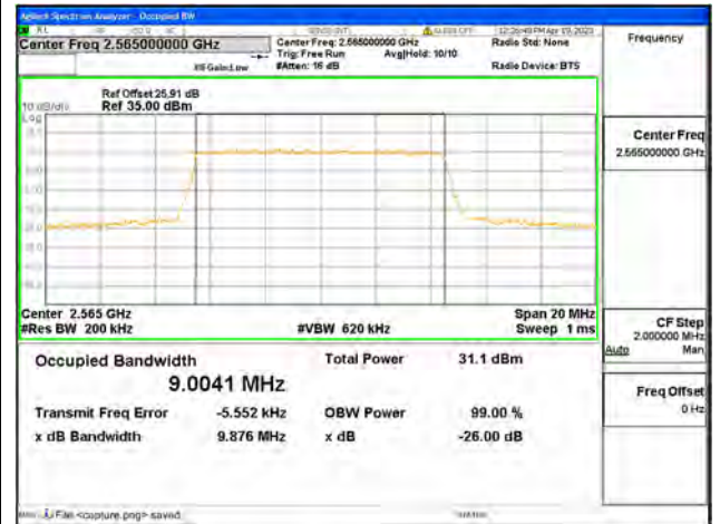
Band7 / 10MHz / QPSK/ High CH
