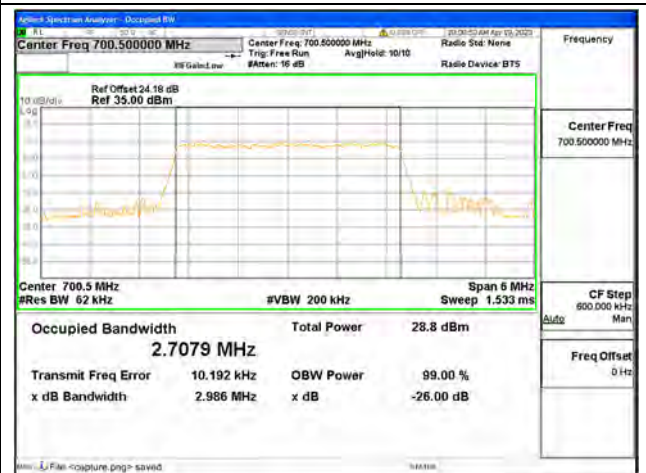
Band12 / 3MHz / 64QAM/ Low CH
