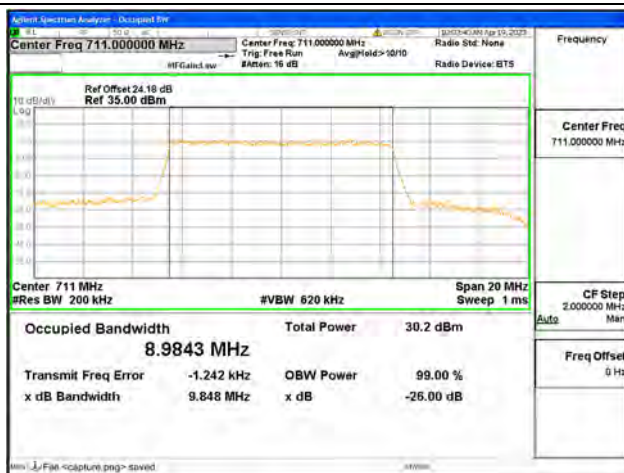
Band12 / 10MHz / 16QAM/ High CH
