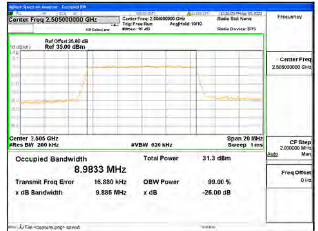
Band7 / 10MHz / QPSK/ Low CH
