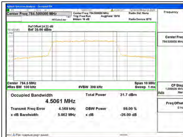
Band13 / 5MHz / QPSK/ High CH
