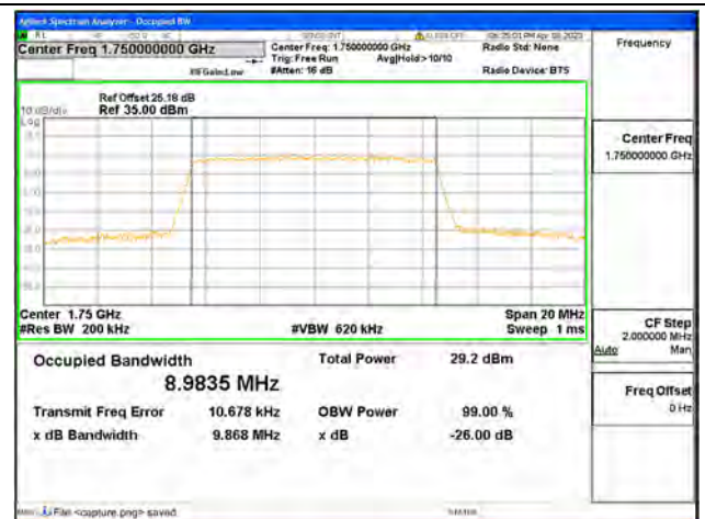
Band4 / 10MHz / 64QAM/ High CH
