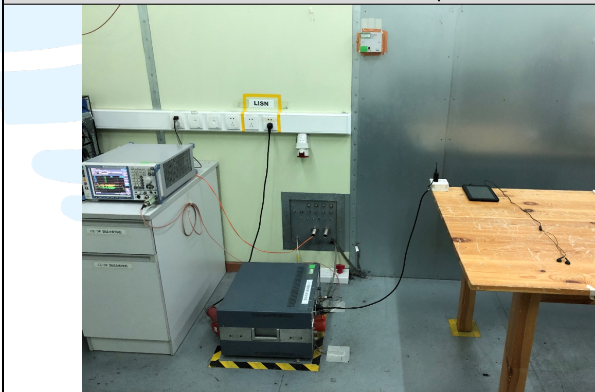
Conducted Emission Test Setup
