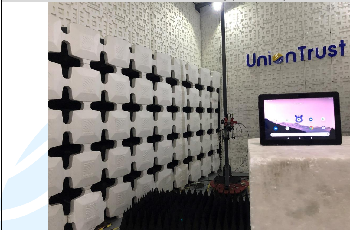
Radiated emission Test Setup (Above 1 GHz)
