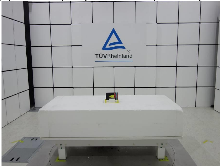
Photograph 8: Test Setup for Spurious Emissions (Back View 1)
