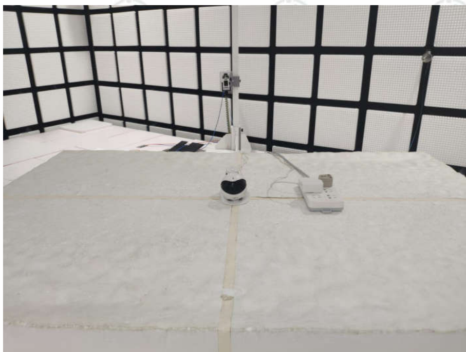
Radiated spurious emission Test Setup-4(Above 18GHz)
