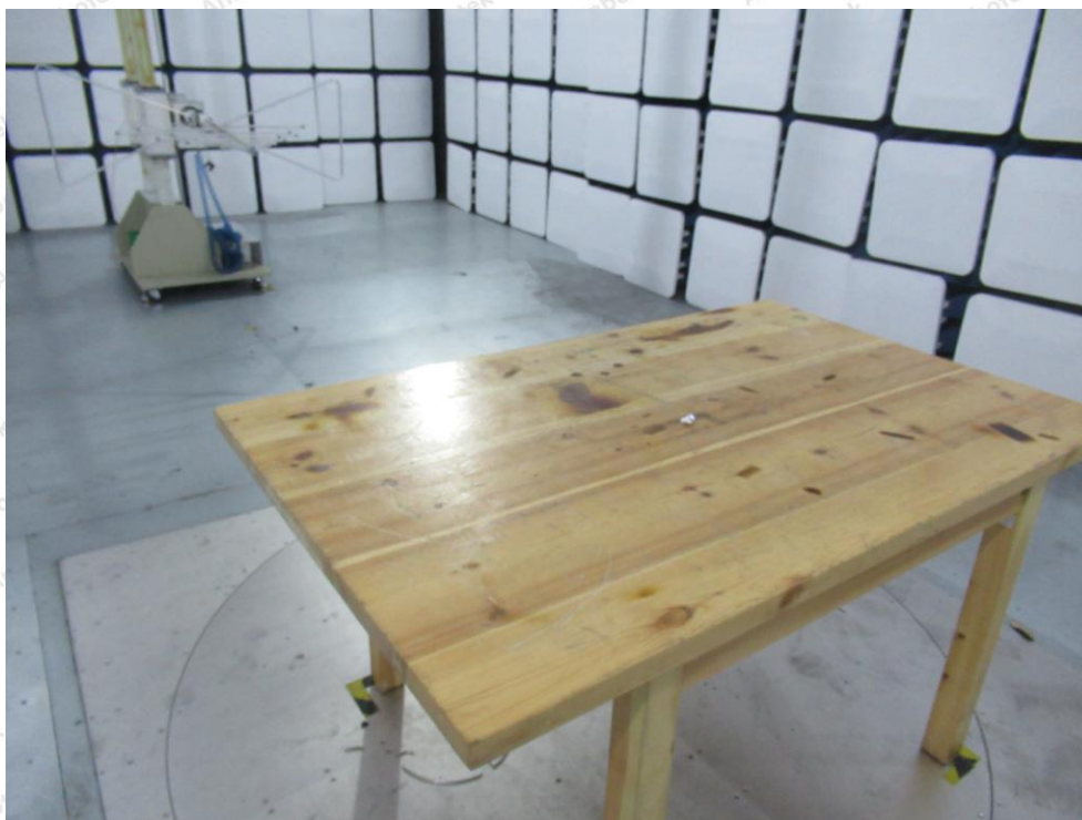
Photo of Radiation Emission Test
