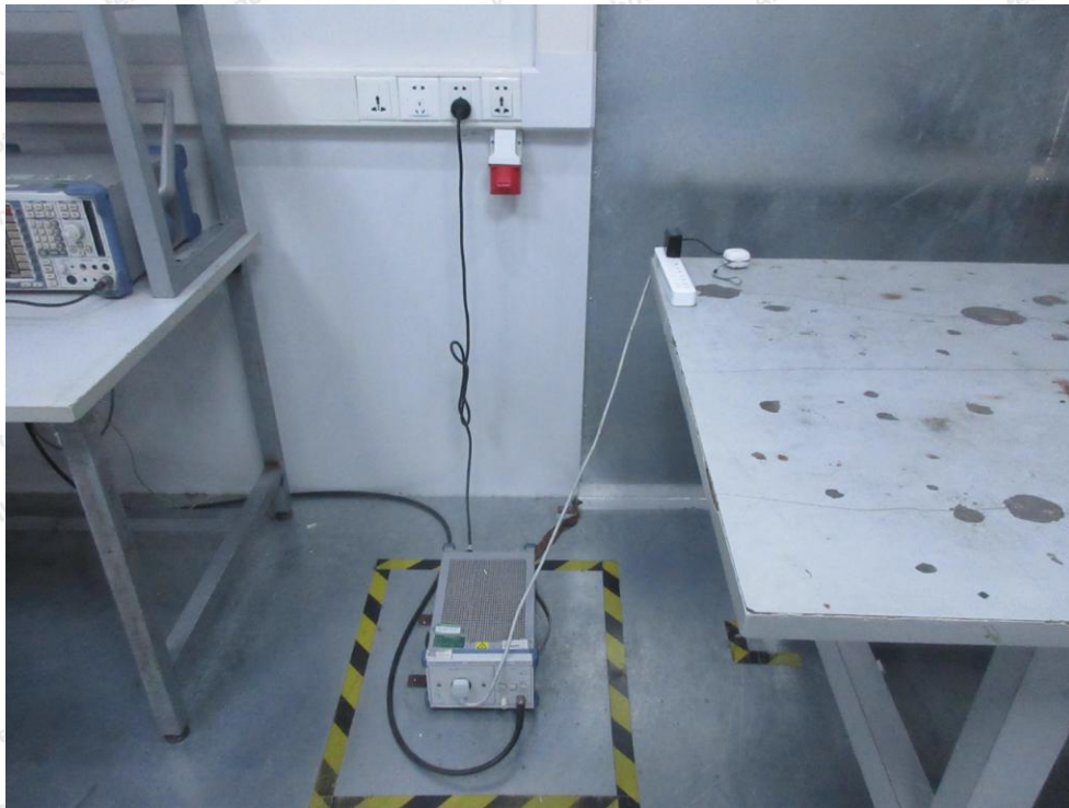
Photo of Conducted Emission Measurement
