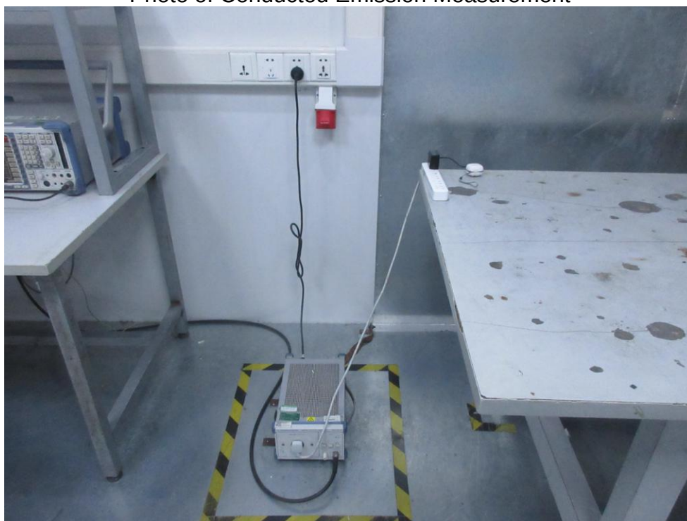
FCC ID: 2AURSFRIENDIE2 Photo of Conducted Emission Measurement
