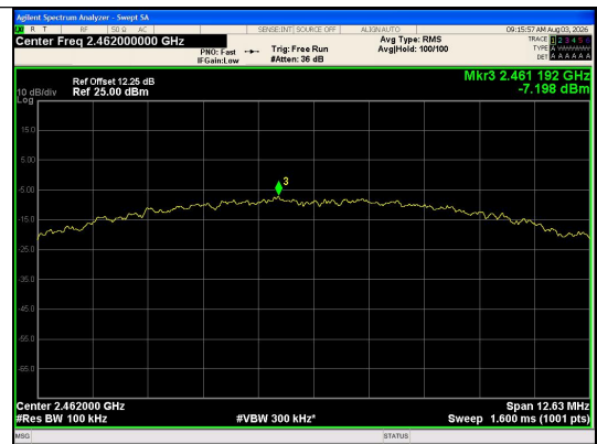
In-Band Reference Level IEEE 802.11b_Channel 11_20MHz_Antenna 0
