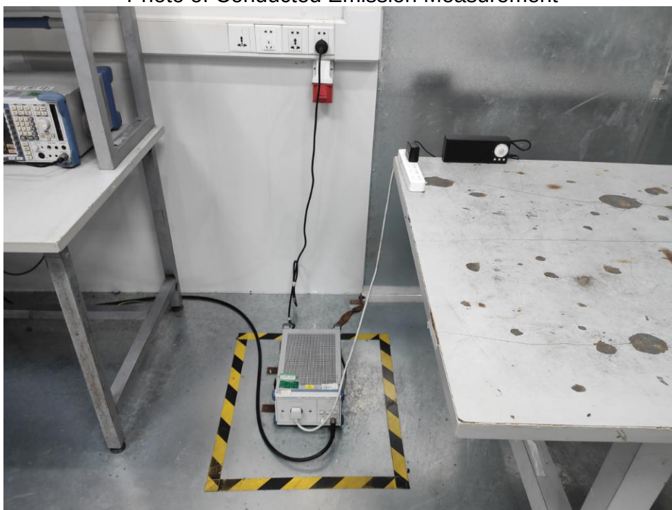
FCC ID: 2AUT6-D23 Photo of Conducted Emission Measurement
